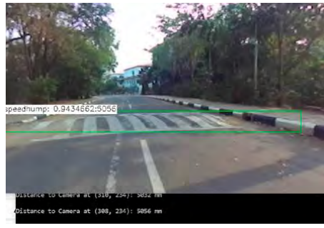
Figure 3. One of the detected Hump at distance of 5.056m [13].
